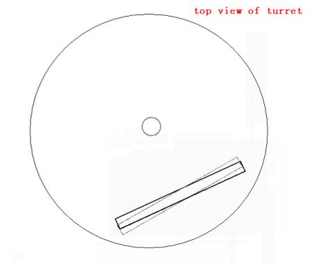
**Roll** This affects how perpendicular the grating grooves are to the system's horizontal axis. The grooves should always be vertical; if they are not, different wavelengths will fall at different heights on the sensor. Typically, roll does not need to be adjusted after moving your Shamrock.
