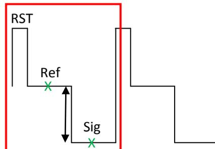
In each pixel (defined by red box) both a reference measurement and a signal measurement are made to determine the level of charge within that pixel. This is done by simply calculating the difference between the measured reference and signal levels. A reset pulse is used at the beginning of each pixel to return the output to a defined level. This technique of Correlated Double Sampling (CDS) is performed digitally by the Field Programmable Gate Array (FPGA).
