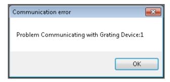
To overcome the issue, the grating and detector offsets will need to be set to zero. In Solis, open the *EEPROM Editor* from *Hardware >> Setup Spectrograph >> EEPROM Editor*.
