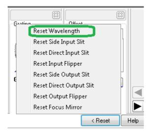
Refer to Technical Solutions document, <u>Shamrock Wavelegth Calibration</u>, to recalibrate the centre wavelegth. In the general case of system crash or power loss, a *Reset Wavelength* operation should also be performed.
