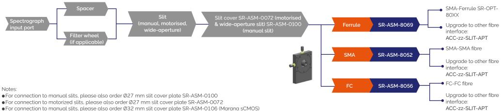
• For connection to motorized slits, please also order Ø32 mm slit cover plate SR-ASM-0107 (Marana sCMOS)
