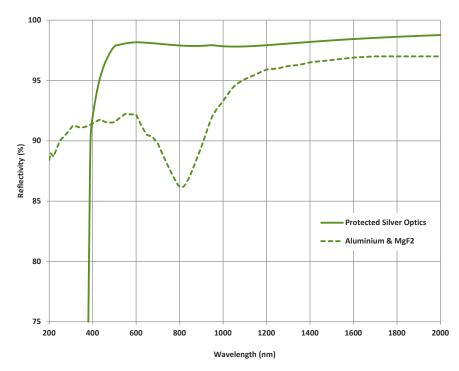
Standard systems use Al + MgF<sub>2</sub> coated optics. Protected silver optics are also available on request for maximum efficiency in the NIR region - recommended for working with Andor iDus InGaAs detectors or IR single-point detectors, such as MCT, PbS and InSb.
